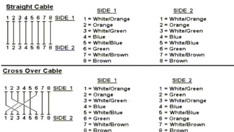
Figure A-1: Straight-Through and Crossover Cable
